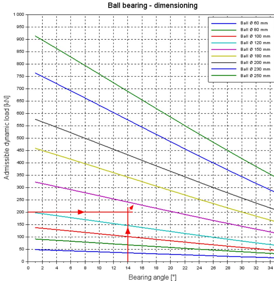
The graphic above shows the possibility of Hagenbuch ball joints. It shows the relationship between the maximum possible bearing angle, the maximum admissible force and the required ball diameter. All possible combinations of force and angle are possible with the standard Hagenbuch construction. Special ball joints can also be developed on request, for example for tight spaces or if the needed tensile and compressive forces are different.
