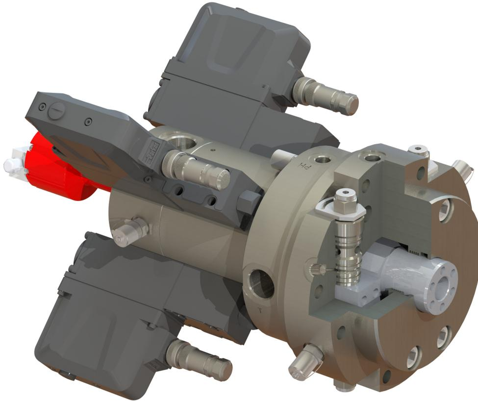
As an option, the hydrostatic anti-rotation device can be fitted on the rod side of a High Performance Shaker. Four hydrostatic bearings prevent the piston rod from rotating. The pressure supply for the bearings is taken directly from the shaker so that no additional hose lines are necessary. The anti-rotation device is centered precisely in relation to the piston rod and does not influence the guidance of the rod.
